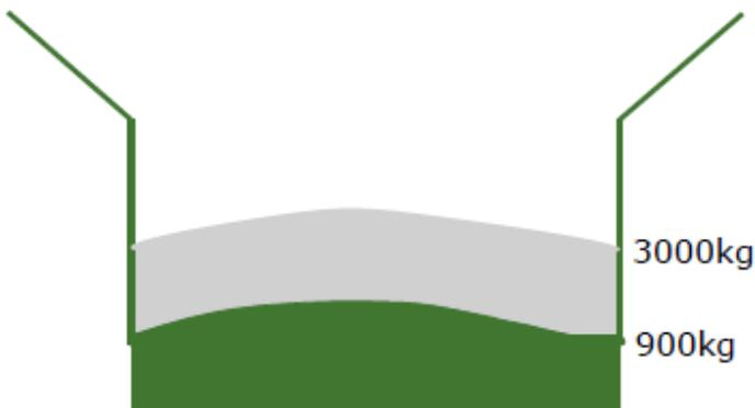
Rate of change of the weight in the grain tank can be estimated with 3 load cells rather than weighing the entire vehicle or grain tank.
