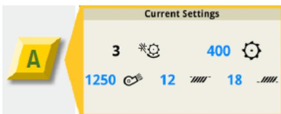
Current settings for concave clearance, rotor speed, fan speed, chaffer clearance and sieve clearance.
